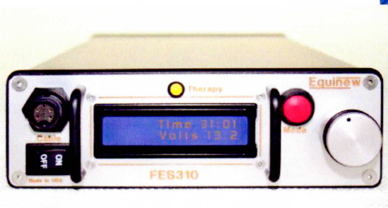
An FES machine delivers computer-generated signals that mimic the body's natural muscle contraction and relaxation. PHOTO COURTESY OF SHEILA SCHILS
